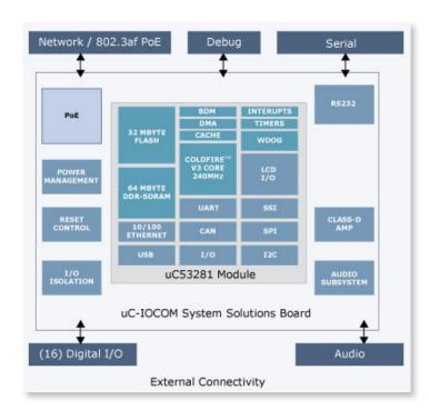
Rugged IP Audio System with Integrated Controls and M2M
