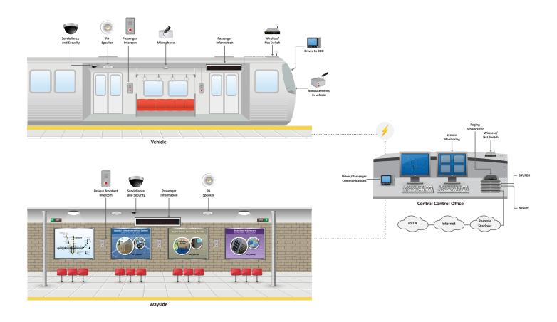
Arcturus transportation system solutions target passenger information, safety, and operator communication in vehicles, stations, wayside systems, central control and airports. They are designed to meet or exceed NEMA recommendations for audio intelligibility and can include central management tools, self-test functions and integration with other systems or equipment.
